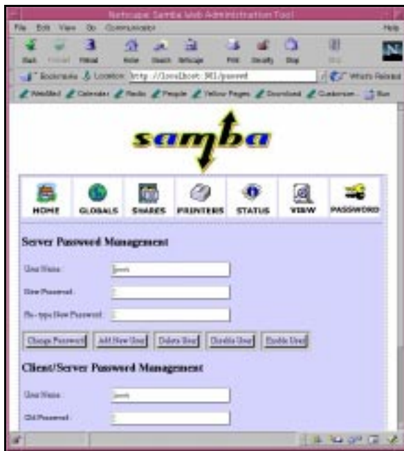
Figure 20. On the Password page of SAMBA you can change the passwords for clients and servers that allow access to the SAMBA file and print services.
