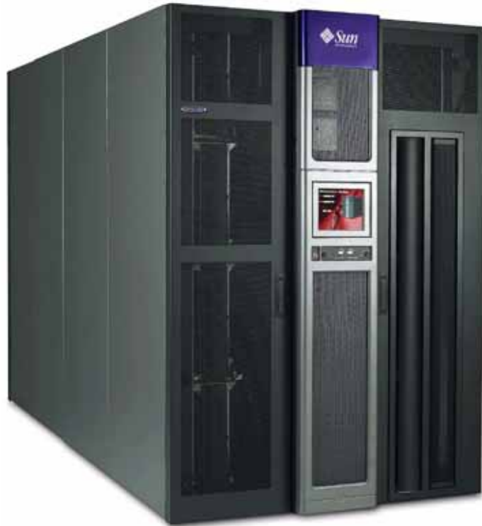
Figure 3. The Sun StorageTek SL8500 library system enables extremely scalable and space-efficient tape archives
