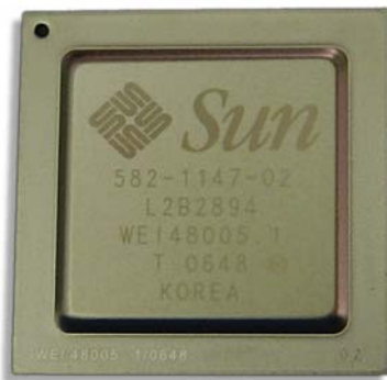
Figure 1-1. Sun's ASIC optimizes I/O throughput for threaded environments
