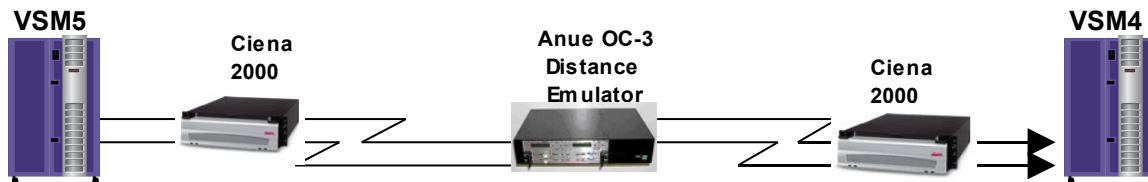
Figure 4: 2 Clink Ciena Channel Extension Configuration
