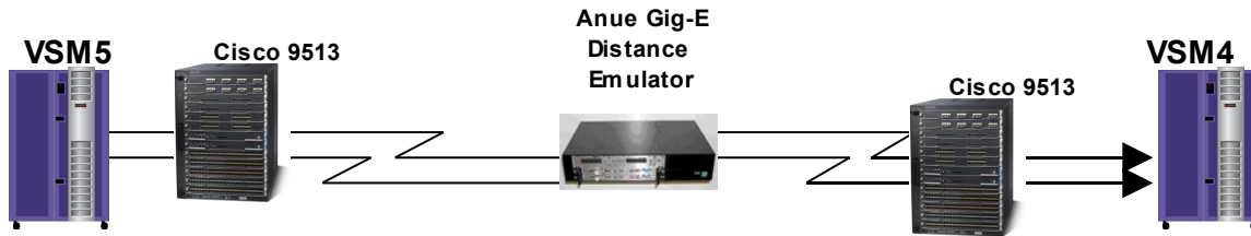
Figure 6: 2 Clink Cisco Channel Extension Configuration
