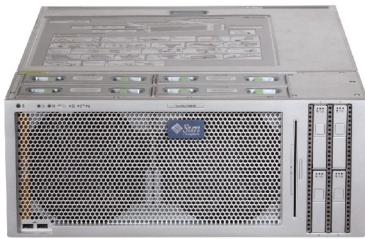
Sun Fire X4600 8 Dual-Core AMD Opteron 885 Processors (2.6 GHz, 1 MB L2 per core) 64 GB DDR RAM
